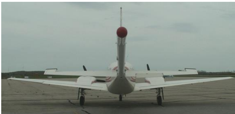
The rigid-boom stinger for the high-sensitivity cesium magnetometer on a Piper PA-31 Navajo aircraft
