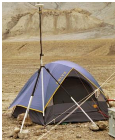
GPS Base Station
