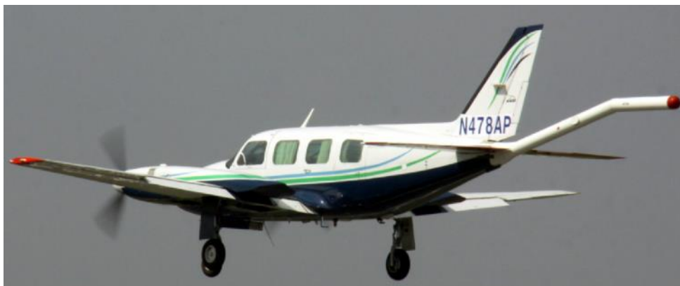
Piper PA-31 Navajo twin-engine survey aircraft - equipped with a GRAV-MAG-EM survey system
