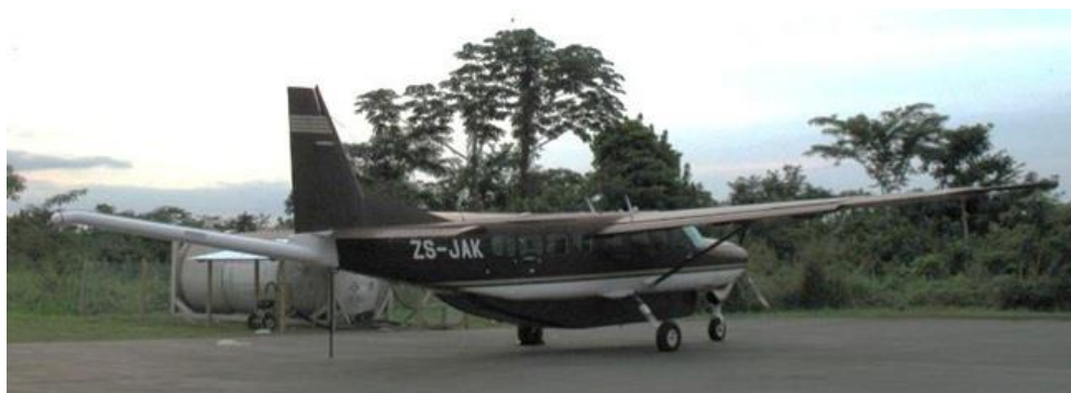
Cessna C208B Grand Caravan turbine engine survey aircraft - equipped with a GRAV-MAG-EM survey system
